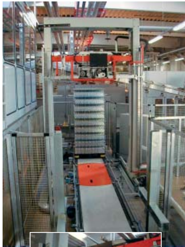
AUTOMATIC VERTICAL STRAPPER (2 straps)
